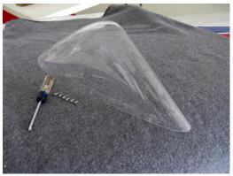
Six sheet metal screws attach the wingtip cover to the carbon fiber skin of the wing. Remove these screws with a small Phillips screwdriver and then remove the wingtip cover. The material is lightweight and should be treated with care. Take precautions not to scratch the light cover or the finish of the wing during this operation. In these photos a soft cloth serves to protect the wing and organize the work.
