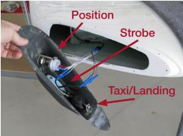
To replace the strobe light, remove the heat shrink material from its electrical connectors and disconnect them. From the outside of the light terminal remove the two sheet metal screws that retain the strobe fixture. Replace the fixture, reinstall the screws, slip new heat shrink tubing over the wiring and reconnect the connectors, then apply heat to the heat shrink tubing.
