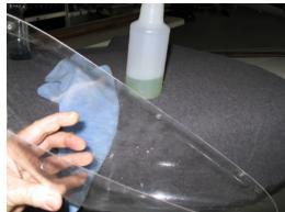
Reinstall the light terminal using the six sheet metal screws. Clean the wingtip cover inside and out with a mild cleaning solution (such as a spray bottle of water with just a few drops of Dawn) and a microfiber cloth. Reinstall the wingtip cover with the six sheet metal screws.
