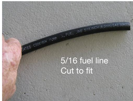
To complete the project, remove the worn snubber and replace it with a new length of fuel line. Reassemble the wheel/inset/bearing components and reattach the nose wheel to the nose gear fork.
