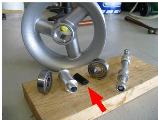
The illustration is excerpted from the Illustrated Parts Catalog for the TL 2000. The snubber is shown in the photo at right, between the inset and one of the wheel bearings.
