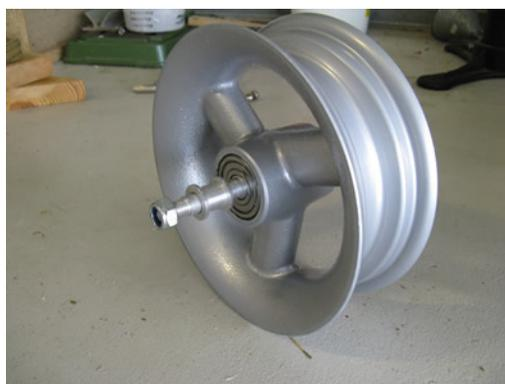
Press or drive the inset out of the bearing (photos below) in order to gain access to the space between the hub and the inset.
