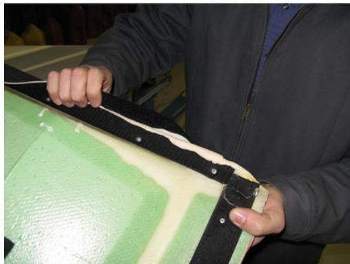
Drill a laterally-centered 3/16" hole approximately 3/4" forward of the lowest portion of the seat, as shown in the inside and outside views, below.
