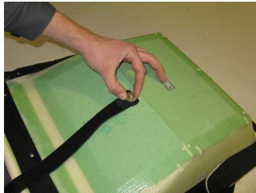
Set the rivet from the inside (top) of the seat, as shown below left. Replace the upholstery using the original velcro. The finished installation is shown below right.
