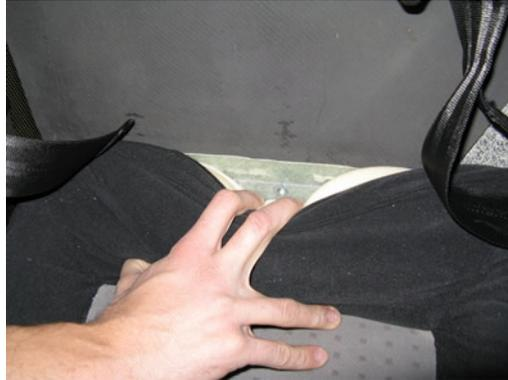
Begin by removing the seat bottom. Five screws attach the seat bottom to the airframe, one at each corner and one in the middle of the back (shown in photo, above right). Pull the upholstery aside to reveal and remove the screws.
