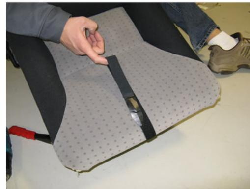
Reinstall the seat bottom using the original screws, taking care not to trap the lap belt retainer beneath the seat. To use the retainer, simply thread it behind the lap belt, cinch down and attach it to itself with the velcro tab. The photos below show the lap belt with and without the retainer in use.
