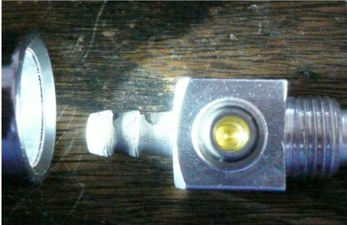
O-ring in proper symmetrical position (This valve has been cut open for better view.)
